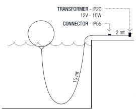
The connector, the transformer and the plug must keep away from the water contact!
